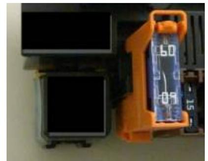
Some component boxes support modular concepts, e.g. the one shown in [figure 1](#). That means the component box can be extended with additional carriers, sockets or smaller component boxes (in a LEGO like way). There are two concepts for modularity: with or without electrical connectivity. If you compare [figure 1](#) with [figure 6](#) you can see, that the relays socket in the lower left corner is mechanically clipped to main component box, electrically it is independent.
