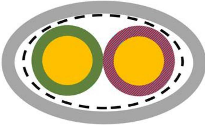
This is an illustration for the multi core example that describes the specification of a multi core wire. The example uses a multi core, which is insulated with a grey insulation, shielded and which contains two FLRY cores of different colouring that are a twisted pair.
